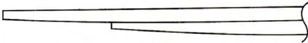
Fig. 3.12 Tapered at the ends of each Leaf
