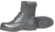
For safety, one should always wear and take care of electrical safety shoes whenever one works in the vicinity of energized equipment's. Unlike regular safety shoes, electrical safety shoes do not have any exposed metal parts. These are specially designed using nonconducting materials to provide insulation from electric shock.
