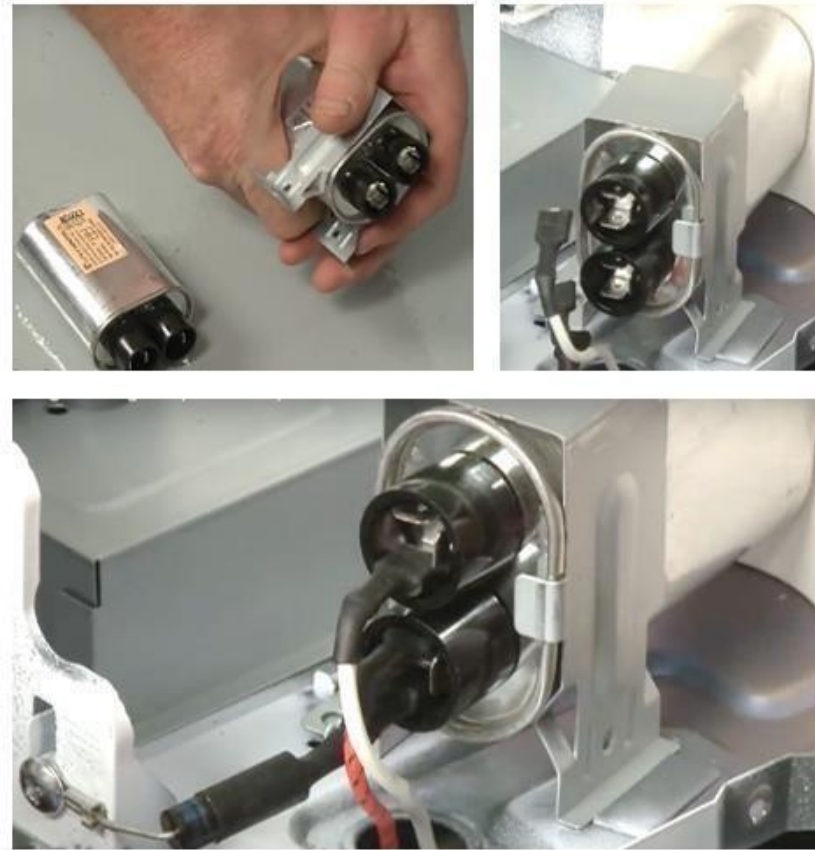
Fig.4.32 Replacing the high voltage capacitor
