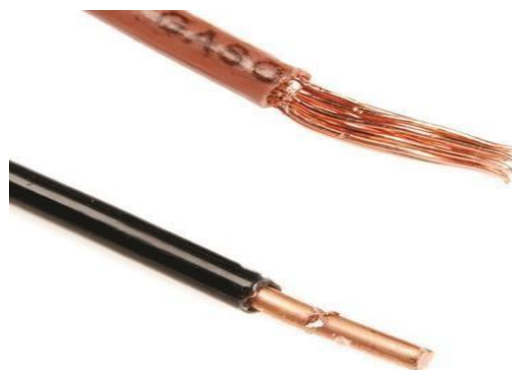
Fig.4.14 Damage on the conductor
