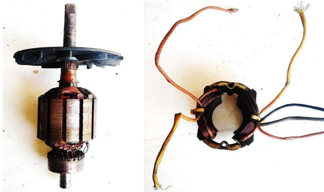
Fig. 3.73 (a) Armature winding (b) Stator winding
