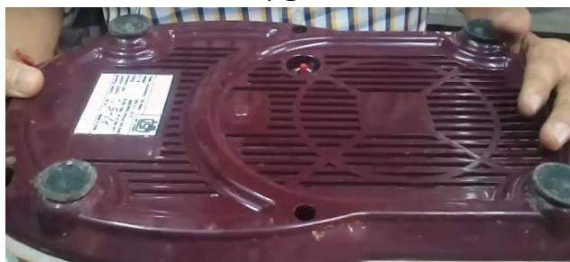
Fig. 3.20: Overload protection button in a mixer/grinder
