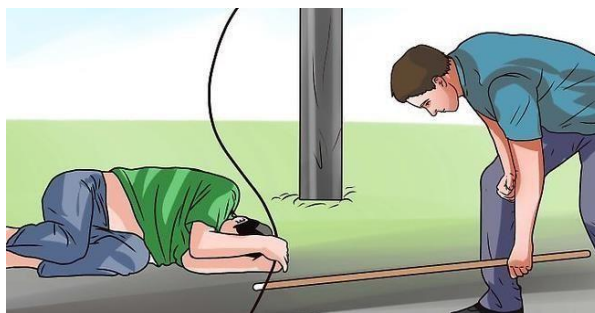
Fig.4.31 Use of non- conductive material to rescue the victim
