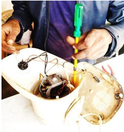
Fig. 3.68: Reassembling of motor
