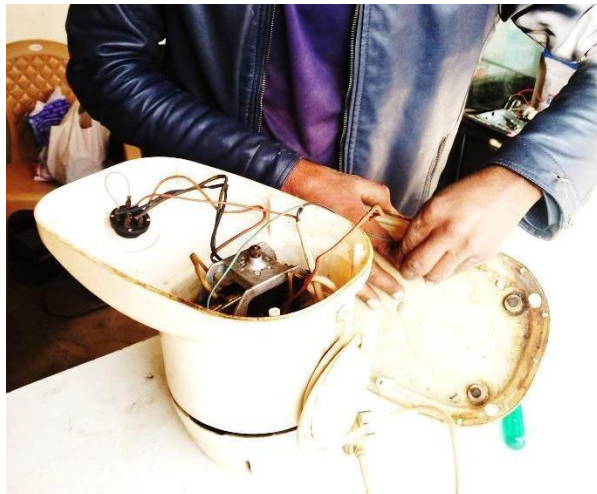
Fig. 3.69 Unlocking the housing of motor
