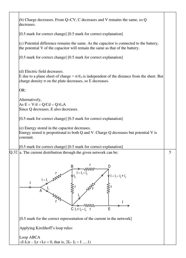
Loop BDCB -(I - I<sub>1</sub> - I<sub>2</sub>)r + I<sub>3</sub>r + I<sub>2</sub>r = 0, that is, I<sub>1</sub> +2I<sub>2</sub>+I<sub>3</sub> = I ---(2)
